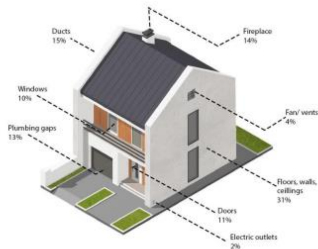
Figure 17 - Energy loss through a building
